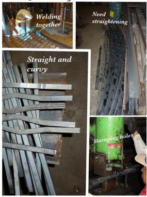
Work continues as you shown in these photos from our visit to the factory. Guards are being welded together shortly they will be shipped to electroplater for their anti-rust treatment. After treatment is completed they go back to the fabricator for a final coating with epoxy paint and are then ready for installation which is scheduled to start around Thanksgiving. We will have an update in our next
